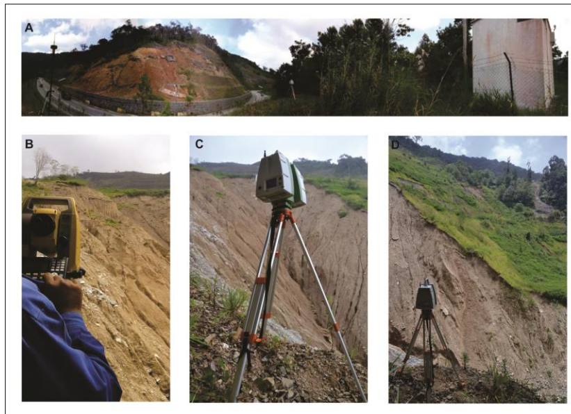
Fig. 1.3: TLSS field campaigns with various laser scanning systems. A) Laser scanner and GPS are used to collect the topographic landslide data. Also, a housing of robotic total station and real-time monitoring system used by PWD. B) Reflectorless total station used in the assessment. C) & D) Leica C10 collecting data over the most active landslide area.
