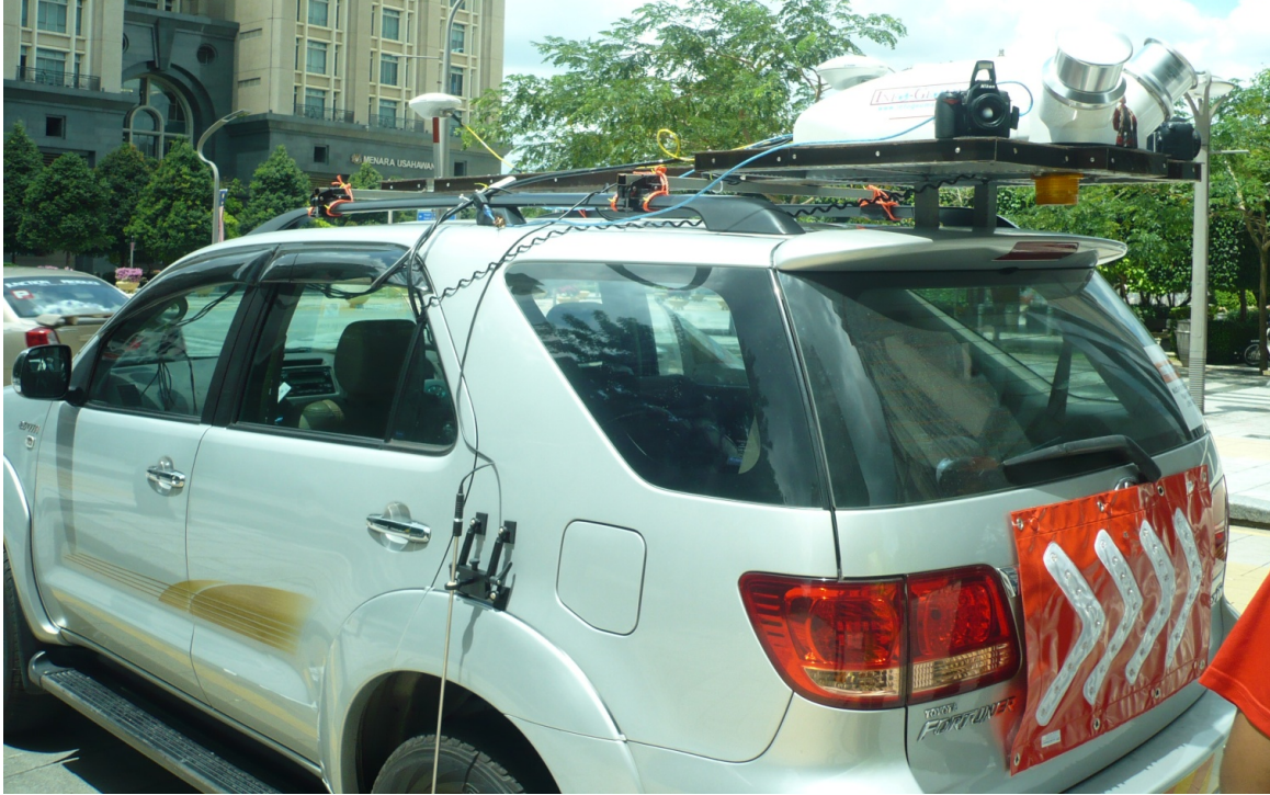
Figure 1: MTLS Dual Laser DynaScan 3 system used
