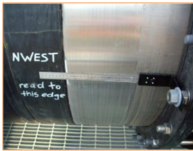
Fixed Ruler at water pipe joint
