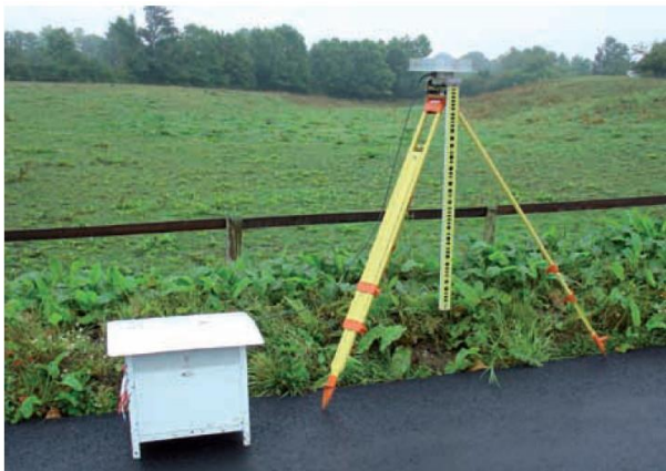
Fig 5: equipment used for ERNIT observations GNSS antenna equipped with a barcode rod and Trimble DINI level
