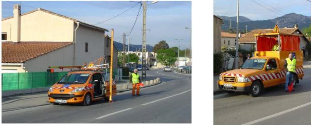
Fig.17: NIREF : motorized precision leveling
