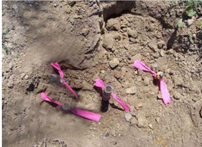
Fig. 4 The ‘Pin Cushion’ Corner (Dietz Surveying, Maryland, USA)
