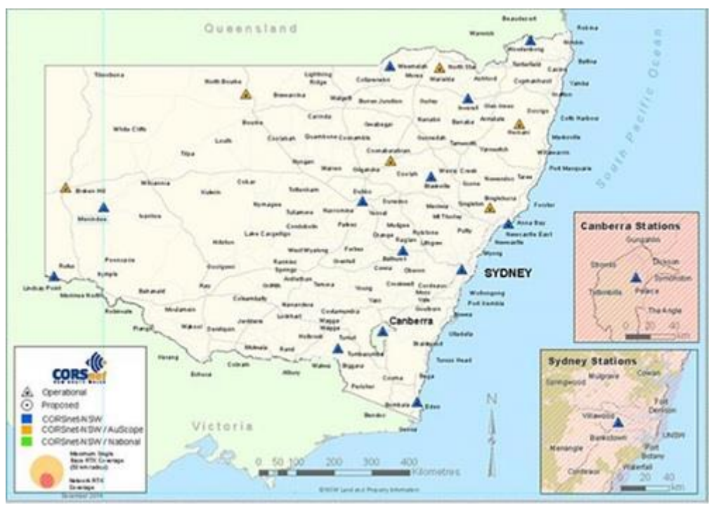
Figure 2: CORSnet-NSW stations capable of tracking Beidou satellites and providing user corrections (as of January 2015). Note that since June 2015, an expanded 61 CORS support Beidou positioning.
