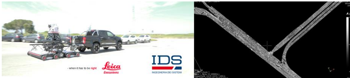
Figure 15 From right to left i) massive array GPR system and mobile laser scanner towed behind a vehicle for network level mapping of utilities ii) Plan view radar tomography time slice of GPR data showing utilities under the ground
