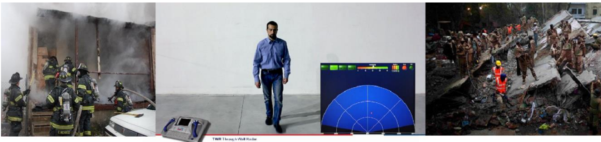
Figure 20 From right to left i) TWR can be used to locate people in smoke filled buildings ii) TWR has simple 2D display which shows person on a screen at a distance of up to 15 metres behind a wall iii) TWR can be used to detect breathing and heartbeat under buried rubble during disaster recovery operations
