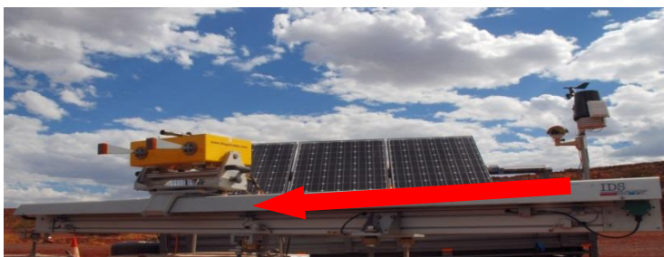
Figure 7a Example of IBIS FL/FM ground based interferometric synthetic aperture radar
