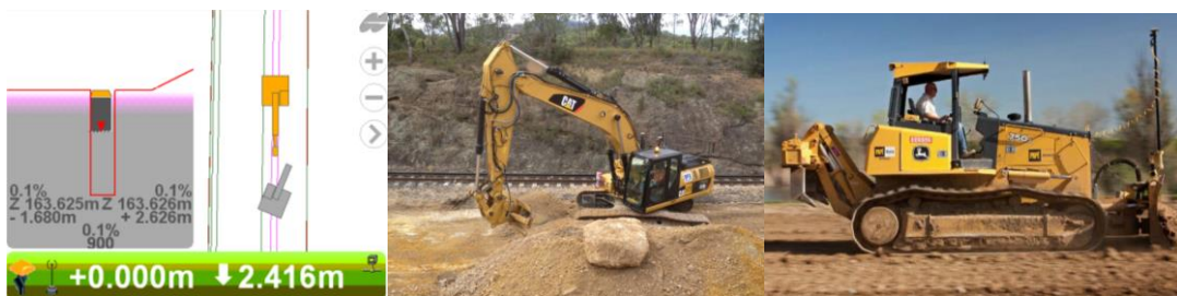
Figure 1. (a) Control screen of an excavator machine control system. (b) Excavator with 3D-GPS system. (c) Dozer with 3D-GPS system. (Position Partners 2015)
