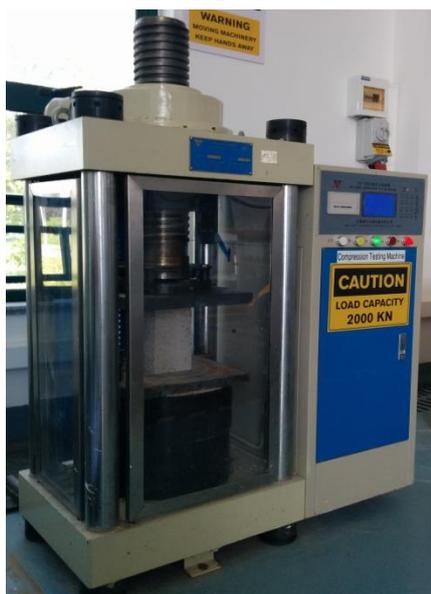
Fig. 6a: Compressive Strength Testing
