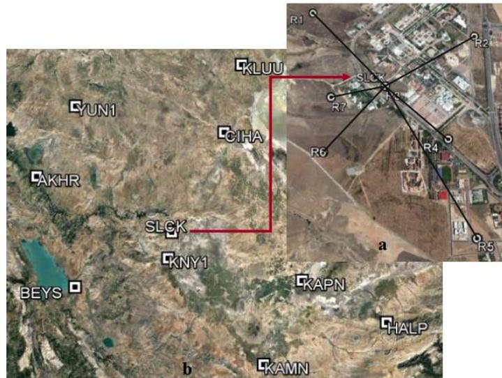
**Figure 1.** Microgeodetic network (a) and Cors-TR stations used in application(b)
