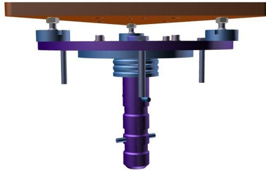
**Figure 6.** Forced-centering element and triangular table
