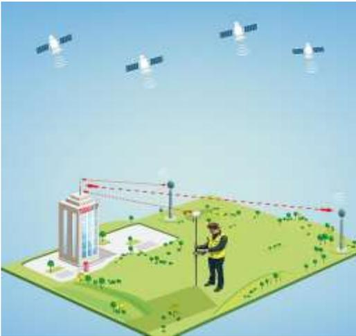
**CORS-Tr Comminicaions:** GNSS Station to Control Center(CC) connections was ADSL and rover user to CC connection was GPRS.
