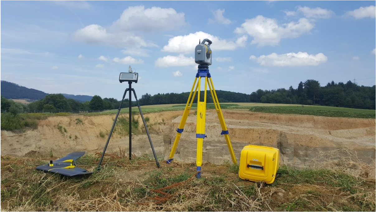
Figure 2: senseFly's eBee Plus UAV (left) with Trimble's SX10 hand controller (center) and SX10 scanning total station with carry case (right).
