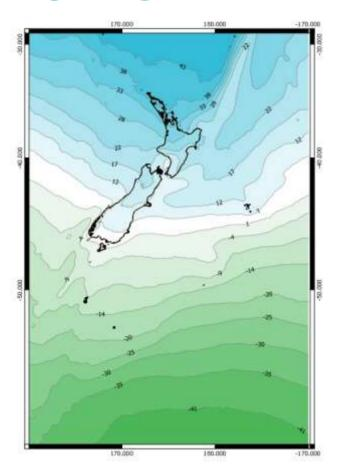
Used to bring orthometric (precise-levelled) and ellipsoidal (GNSS) height differences into a consistent reference frame
