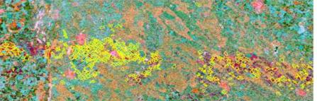
LPIS blocks of claims of damages and damages detected by the analysis of radar satellite images are coincided well Analysis were carried out within 10 days after the storm (including satellite image purchasing)
