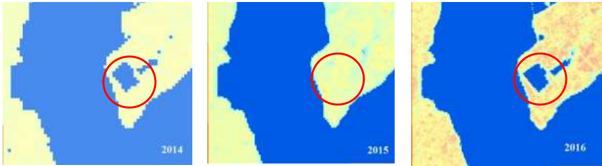
Figure 10. Natural color composite images (above) and MNDWI index images (below): Vegetation covers the lake surface in 2015 so the MNDWI index image does not extract lake surface water; Observing natural images and MNDWI index images of 3 years 2014, 2015, 2016 we can extract the surface water of that lake
