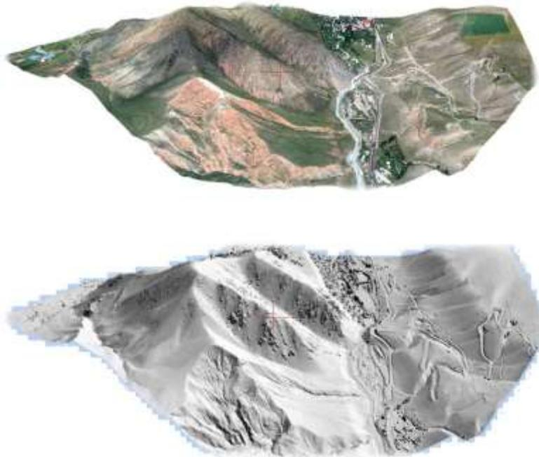
Figure 6: 3D point cloud and DTM
