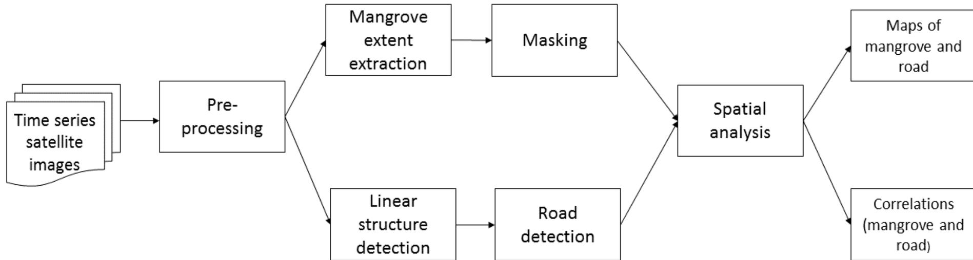
The SPEAR Lines of Communication (LOC) – Roads tool ([Wollmer, 1970](#)) in ENVI software was used to highlight roads to aid manual digitizing of the road system.
