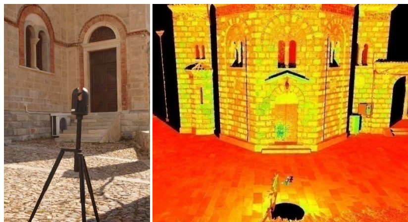
Figure 3: Snapshot of the scanning process (left) and example of a point cloud output (right).
