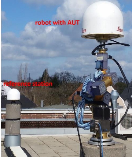
Figure 2: Calibration set-up at IfE. In the foreground the robot with the AUT can be seen. At a distance of approximately 8 m the reference station is located.
