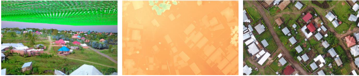
Figure 4: Data products derived from UAV images. A: 3D point cloud; B: digital surface model; C: orthophoto
