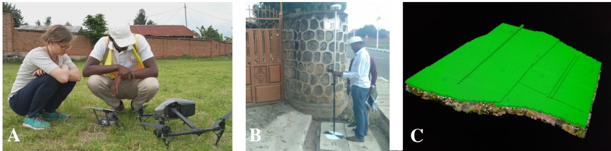
Figure 2: UAV data collection. A: checking the UAV DJI Inspire Pro before the flight; B: measurement of ground control points for georeferencing; C: data processing in Pix4D
