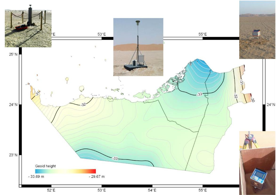
Figure 1: hybrid gravimetric geoid. Values in m. Contour interval is 20 cm
