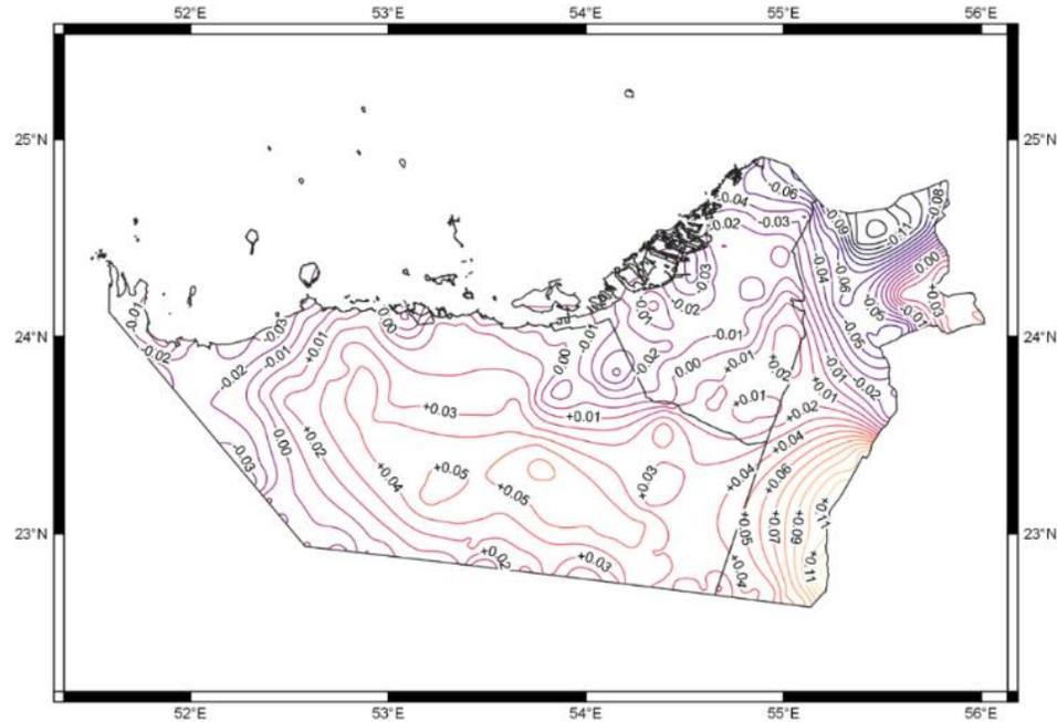
Figure 13: Contour lines of the LSC adaptation surface (values in meter). Corrections range from -13.3 cm to +13.6 cm
