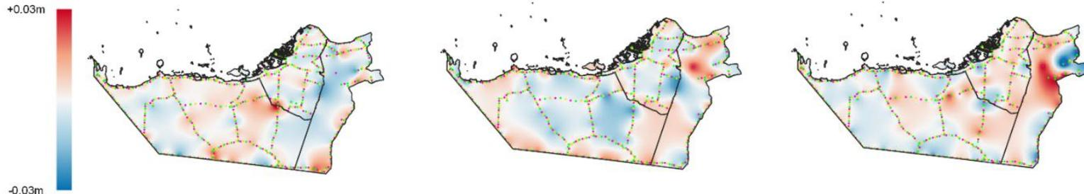
Figure 12: Comparison between LSC surface created with all GNSS-Levelling benchmarks and with subset 1, 2, and 3
