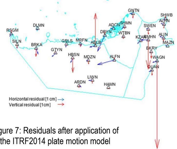
Figure 7: Residuals after application of the ITRF2014 plate motion model
