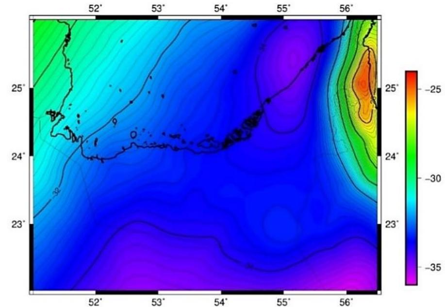
Figure 9: Gravimetric geoid. Values in m. Contour interval is 20 cm
