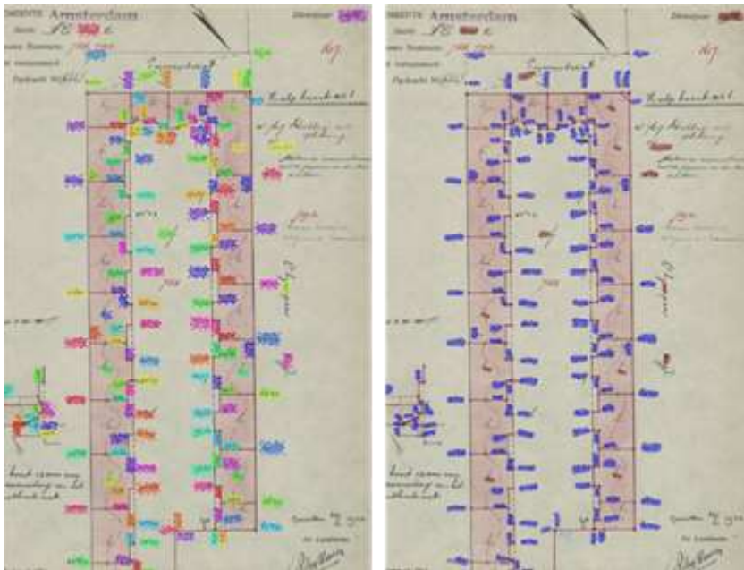
Figure 6: The Mask-RCNN model applied to a field sketch (left). After post-processing (right), blue-coloured masks are associated to a line and point, and red-coloured masks are disregarded.
