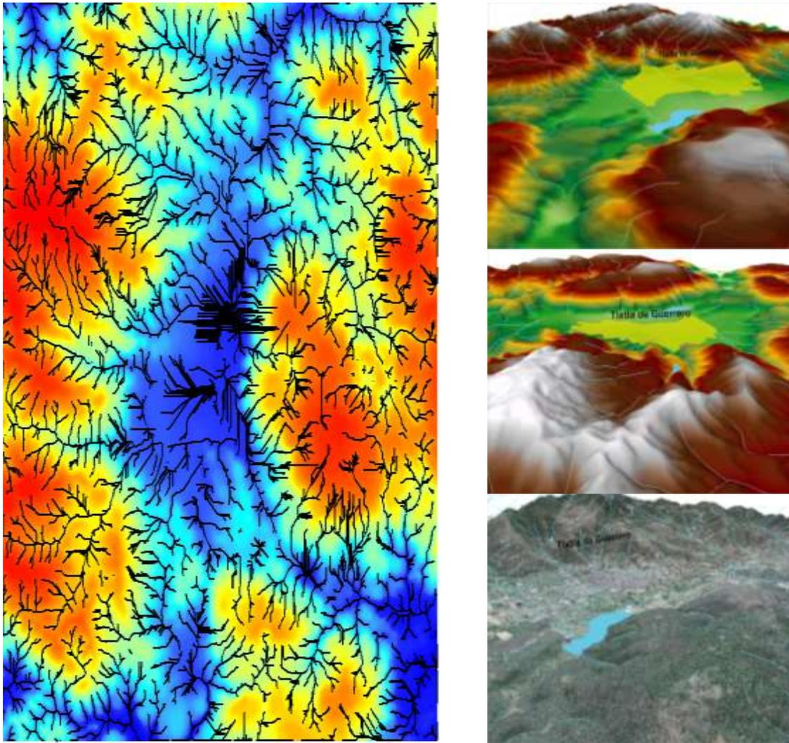
*Figure 8. Digital terrain model and derived riverbeds with a flow accumulation parameter of 100 cells and its result of 8,544 segments that make up the network. On the right is the digital 3D elevation and orthoimage model with the geographical location of the town of Tixtla.*
