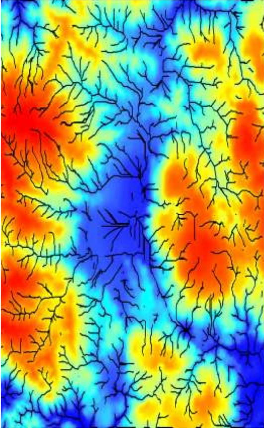
Digital terrain model and derived riverbeds with a flow accumulation parameter of 400 cells resulting in a network consisting of 1,919 segments.
