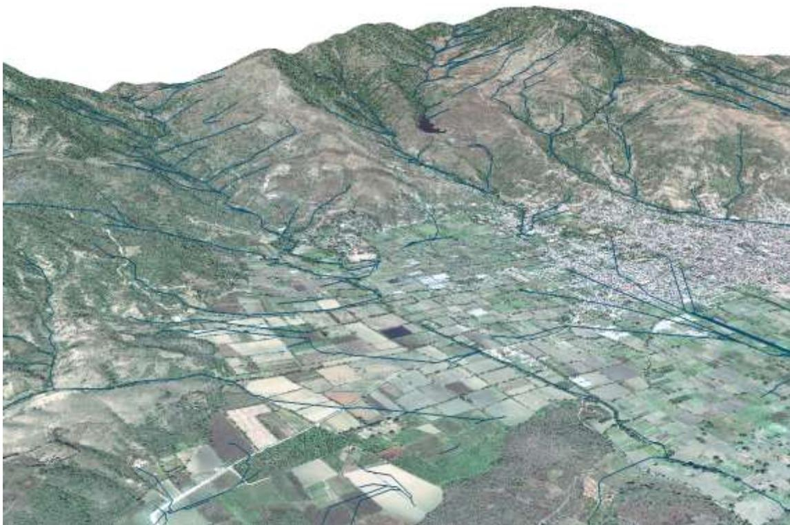
*Figure 10. 3D modeling in a GIS showing the orthoimage and network of riverbeds generated from the digital terrain-type elevation model with a flow accumulation parameter of 100 cells and its result of 8,544 segments in the Tixtla area.*
