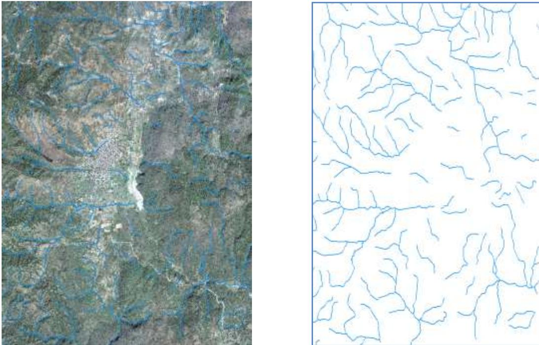
*Figure 5. In the image on the left the orthoimage with the riverbeds of rivers and digitized streams both overlapping in the GIS. In the image on the right the result obtained from the riverbeds near the town of Tixtla*
