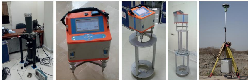
Figure 3 : Absolute and relative gravity survey. Left: FG5 absolute gravimeter. In the center: CG6 measurements of the vertical gradient of gravity. Right: GNSS and CG5 relative gravity combined.
