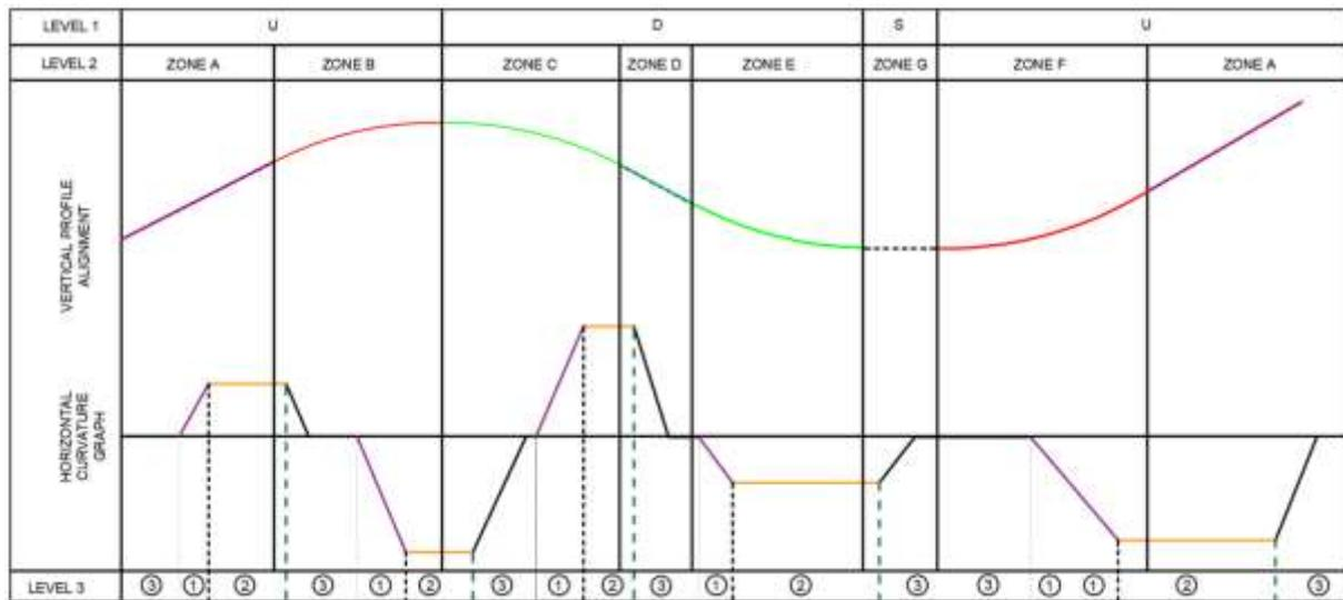
Fig. 2: Formulation of the roadway segmentation hierarchy levels using the vertical roadway alignment and the horizontal curvature graph.
