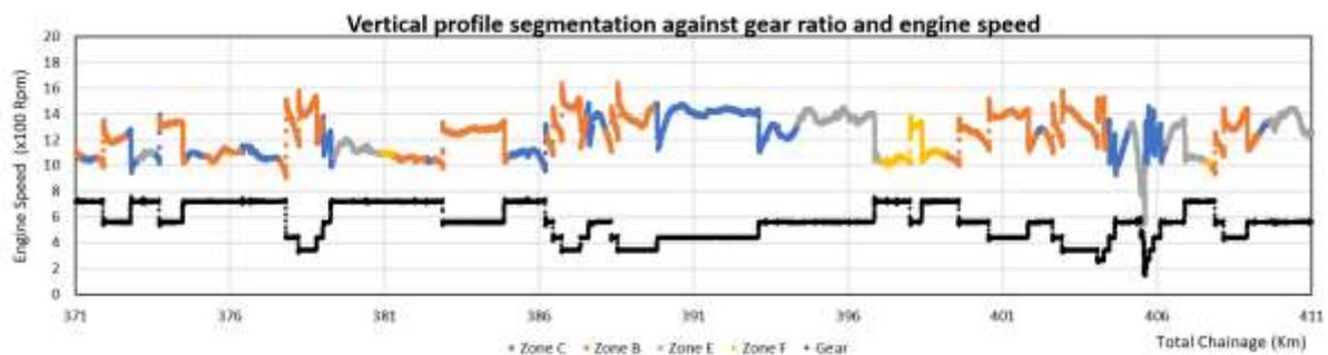
Fig. 11: Vertical profile-based segmentation for the selected trajectory VS gear ratio and engine speed
