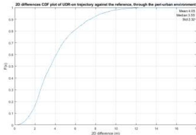
Fig. 5: 2D differences of UDR-on trajectory against the reference
