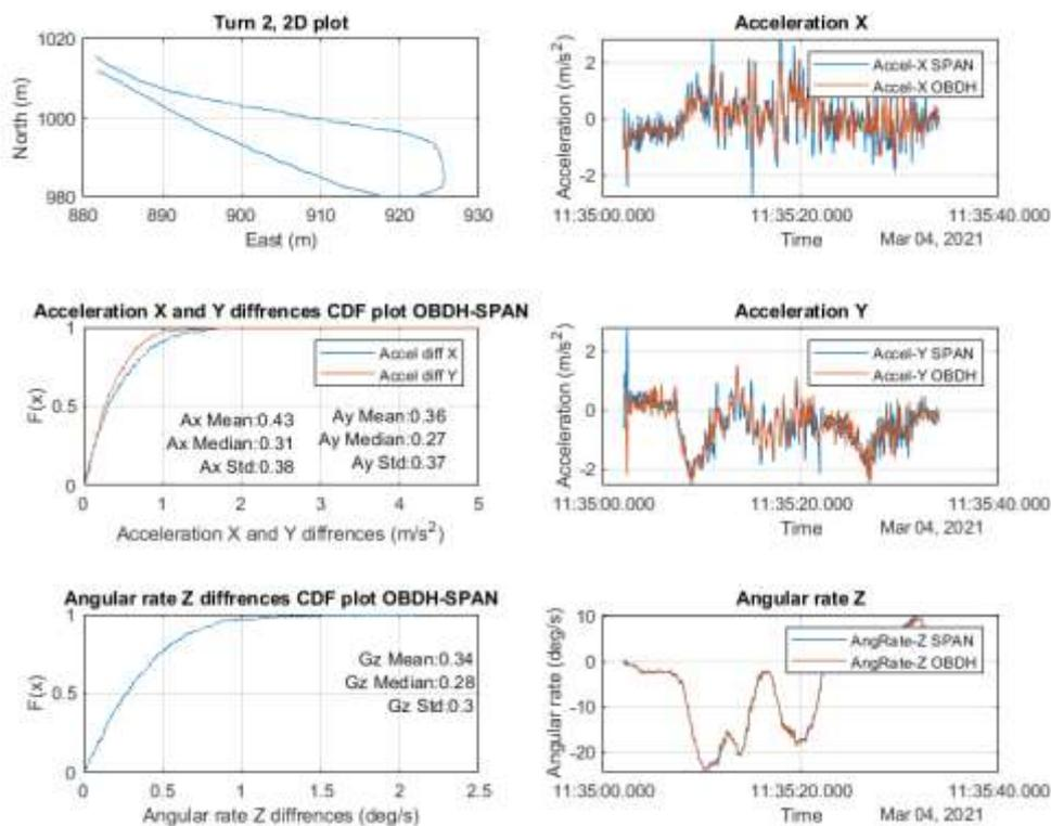
Fig. 9: IMU quality statistics for a sharp left-turn
