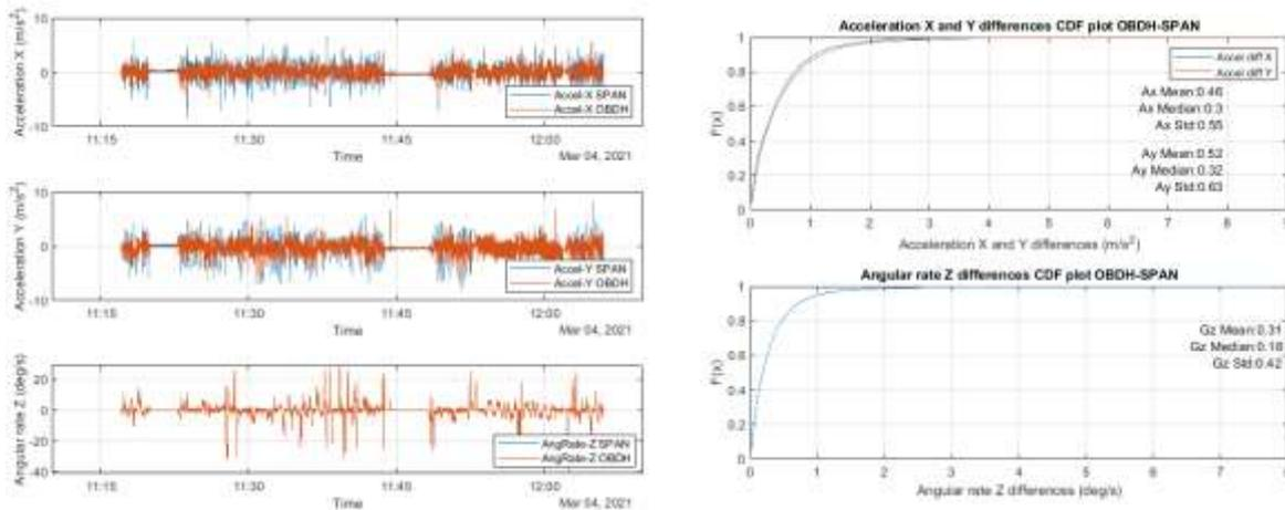
Fig. 8: Acceleration X, Y and angular rate Z timeseries (left) and corresponding differences CDF plots (right).
