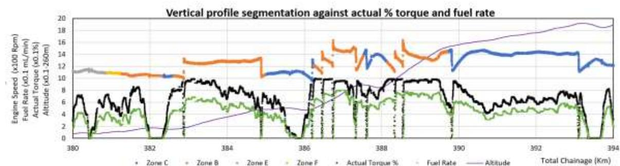
Fig. 12: Vertical profile-based segmentation for the selected trajectory VS actual torque % and fuel rate
