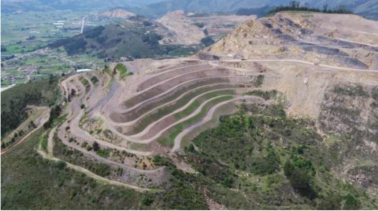
Figure No. 4 Progress of the rehabilitation process Sterile disposal area Belencito Mine
