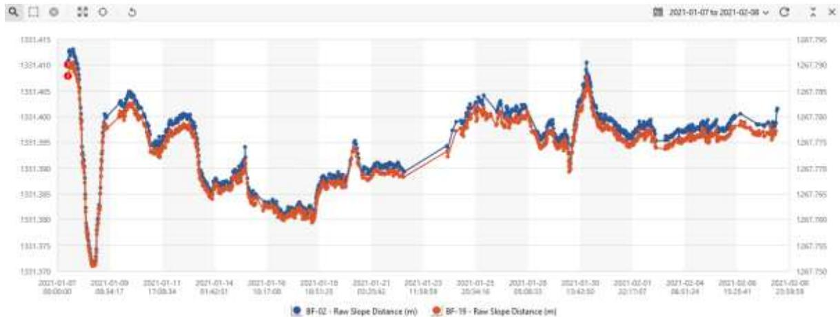
**Figure 13** Slope distance measurements on BF-02, BF-19 points in the period from January 7 to February 8
