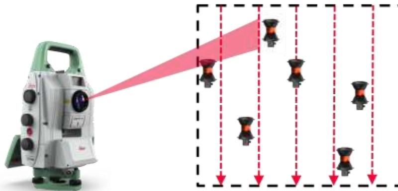
**Figure 5** Leica TM60 conducting the prism search within a defined area. The configuration was done using GeoMoS AutoLearn feature.
