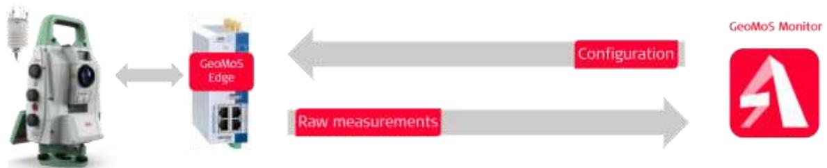
**Figure 6** Measurement process with GeoMoS Monitor and GeoMoS Edge
