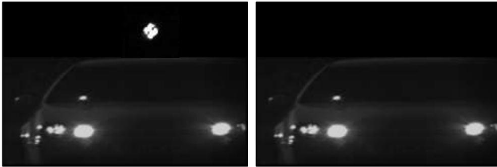
**Figure 4** Bright (left) and dark (right) ATRplus image of a car and a reflective prism
