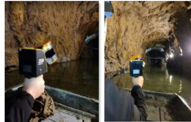
Fig. 5. Measurement with a GeoSLAM ZebHorizon in the Włodarz Complex. Source: own archive.
