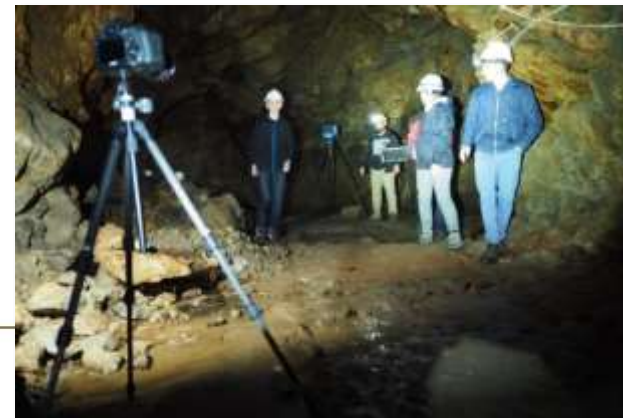
Fig. 6. Measurement with a TLS methodology in the Włodarz Complex. Source: own archive.
