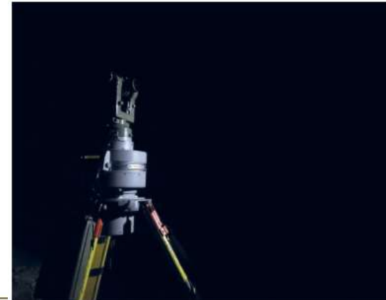
9. Underground giroscopic measurements. Source: own archive.
