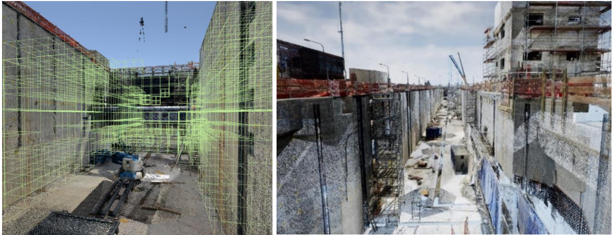
Figure 3: Underlying octree -green- to increase performance (left); Example of a large point cloud being rendered in our VR system (right).
