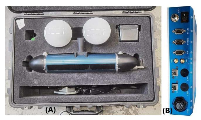
Figure 1. (A) 3DSS-IDX-450 Sonar with GNSS. (B) Sonar Interface Unit (SIU) powers the sonar head and has an integrated
