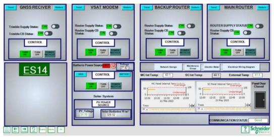
Figure 4: GeoSCADA monitoring for KSA-CORS
