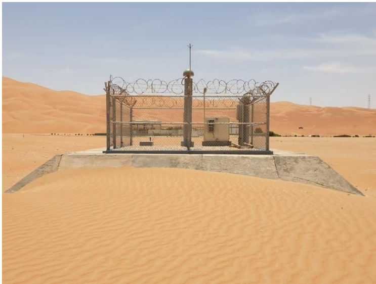
Figure 7: KSA-CORS High Monumentation Base at the northern edge of Rub' Al Khali
