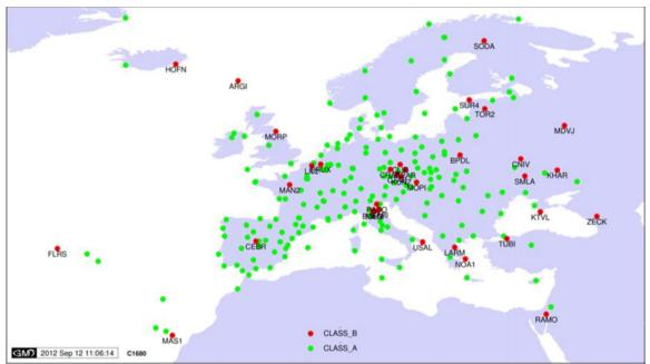
Fig. 2 EPN site categorization, status Oct. 2012. In green: Class A stations; in red: class B stations.
