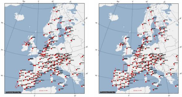
Fig. 5 Difference between official ETRS89 coordinates adopted in the different countries and the latest EPN cumulative coordinate solution
