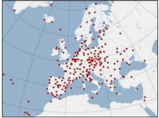
Fig. 1 EUREF Permanent GNSS Network (EPN), status Oct. 2012
