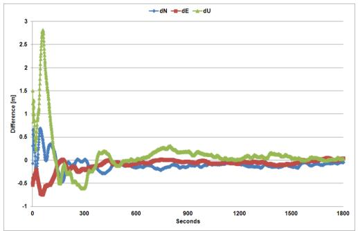
Fig. 3 Differences of real-time coordinates using the BKG Ntrip Client (BNC) with ETRS89related satellite and orbit corrections for station ZIM2 w.r.t. the ETRS89 coordinates
