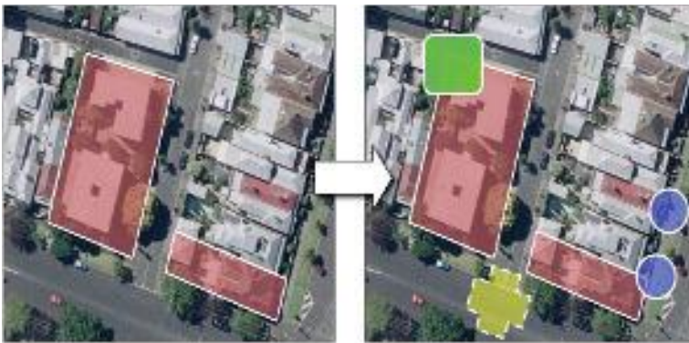
◀ Figure 2, Cadastres will change from purely parcel-based systems (left) towards systems of layered property objects.
