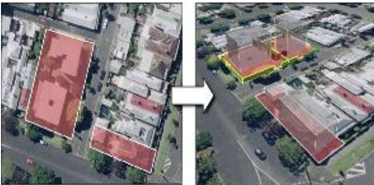
◀ Figure 3, Cadastres will expand from 2D approaches (left) to include 3D (right) and 4D perspectives.
