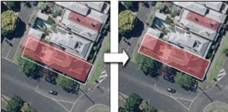
◀ Figure 1, Cadastres will move from approximate boundary representation (left) towards survey-accurate boundary representation.
